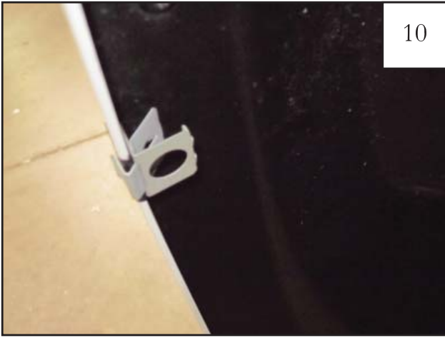
Center clips on the tabs installed in Step 8 and push onto the bumper cover.
