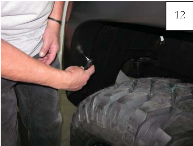
Reposition flare on fender. Using a #2 Phillips, start a supplied Screw (SW1-0058) through two forward hole locations and through each Clip installed in step 10. If needed, use scratch awl to locate holes.
