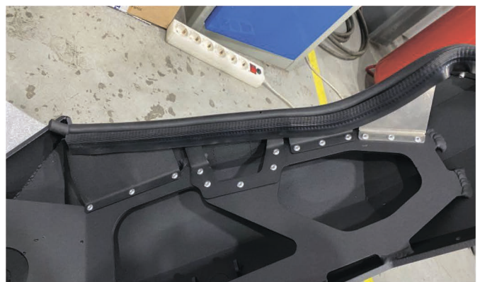
42. Put the seal on the bumper.
