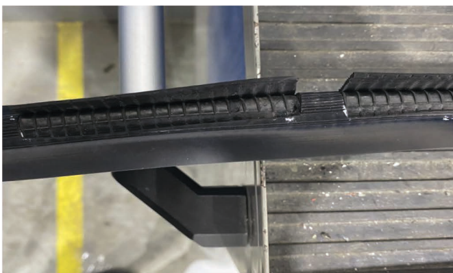
41. Remove the reinforced section of the seal.
