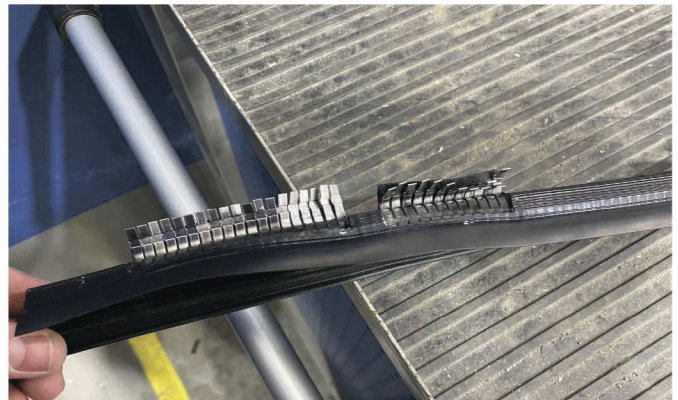
40. Bend the reinforcement of the seal where cut.
