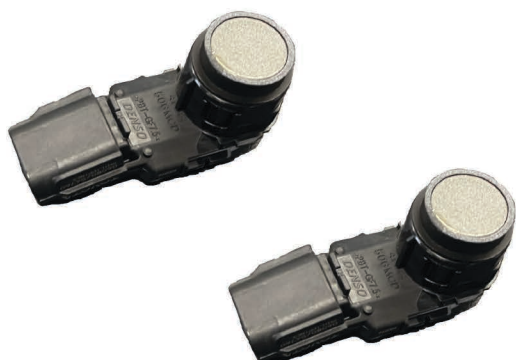
27. Remove parking sensors from factory bumper.
