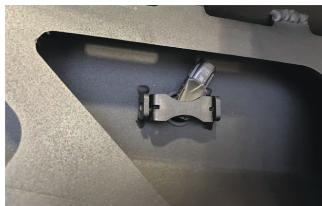
30. Put parking sensor in bumper body and fix them, using parking sensors holding brackets (pos.11), screw M6x20 (pos.G) and washer 6mm (pos. L).
