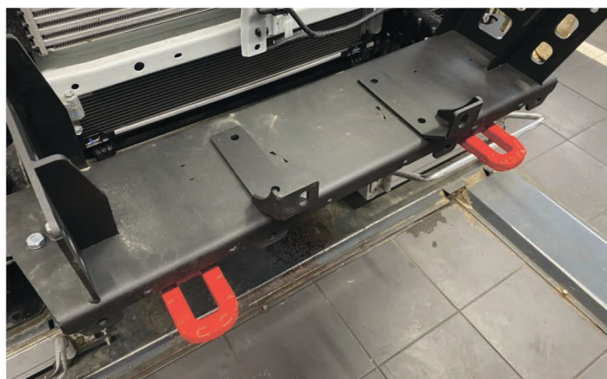
25. Fix left and right winch fairlead brackets (pos.20, pos.21) on winch bracket.
