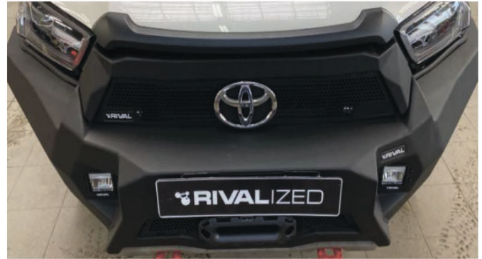
62. Install the emblem badge on grill surface (pos.2). Install grill (pos.2) on brackets (pos. 12-15), using screw M6x20 (pos. G) and washer 6mm (pos. L).
