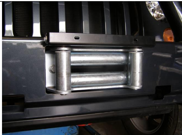
Roller Fairlead installed
