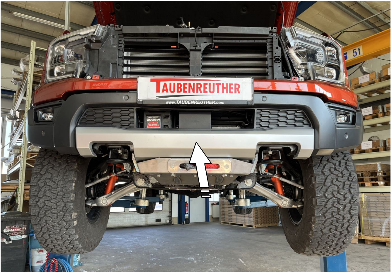
43 Untere Blende wieder montieren / Mount the lower cover again!
