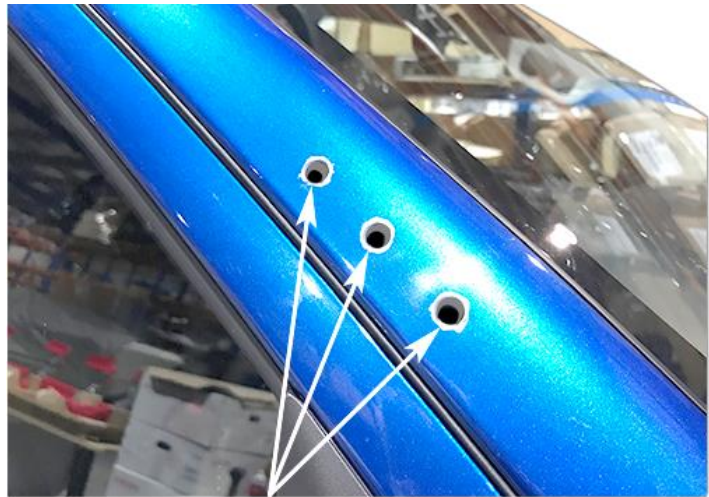
Drill A-Pillar Panel 8mm, Inner Panel 6.5mm
