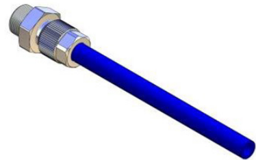
C. Feed the nut up to the connector, fully tighten by hand and finally tighten one additional turn using spanners
