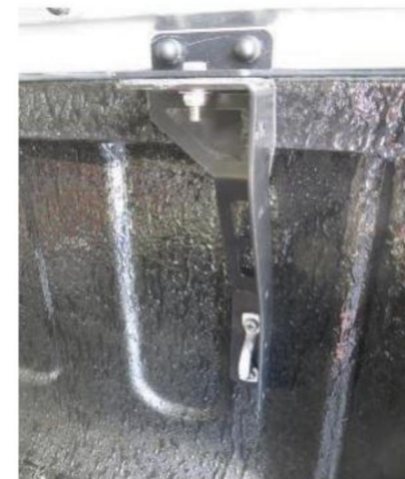
Figure 18.2: Rear-Right Support Bracket Installed
