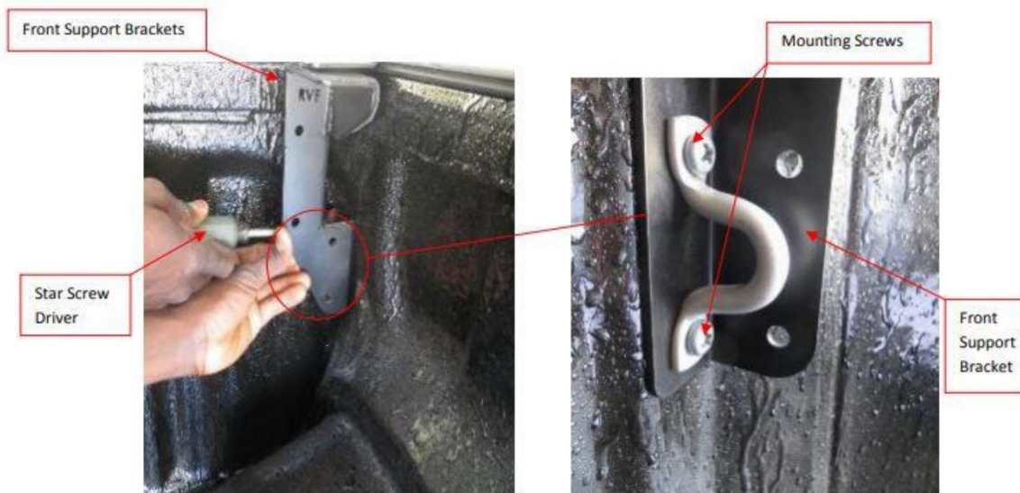
Figure 7: Installing Front Support Bracket
