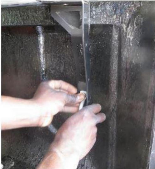
Figure 8: Aligning the Rear Support Bracket
